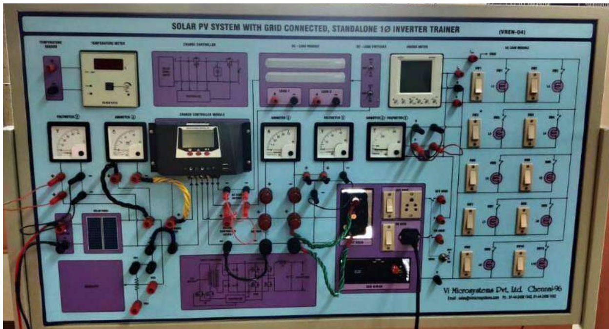
Photovoltaic cells control unit
