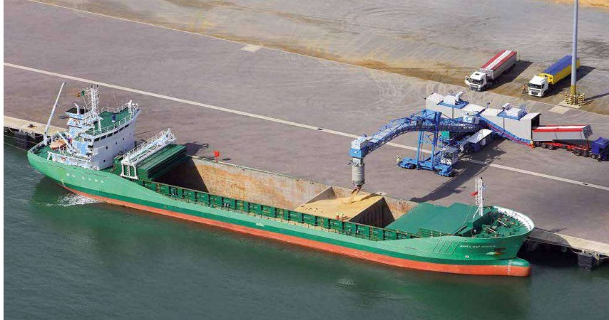
Independent Mobile Material Feeder feeds an existing ship loader
